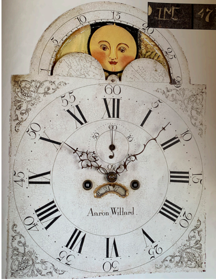
Fig. 7. 12 inch Aaron Willard tall clock moon dial with floral corners and raised gesso gilt borders, transfer printed small “half map,” hemispheres, signed “J. Minott / No. 222” on rear upper left, signed on front “Aaron Willard.” in print lettering. Courtesy of Gary R. Sullivan Antiques, Sharon, Mass.
